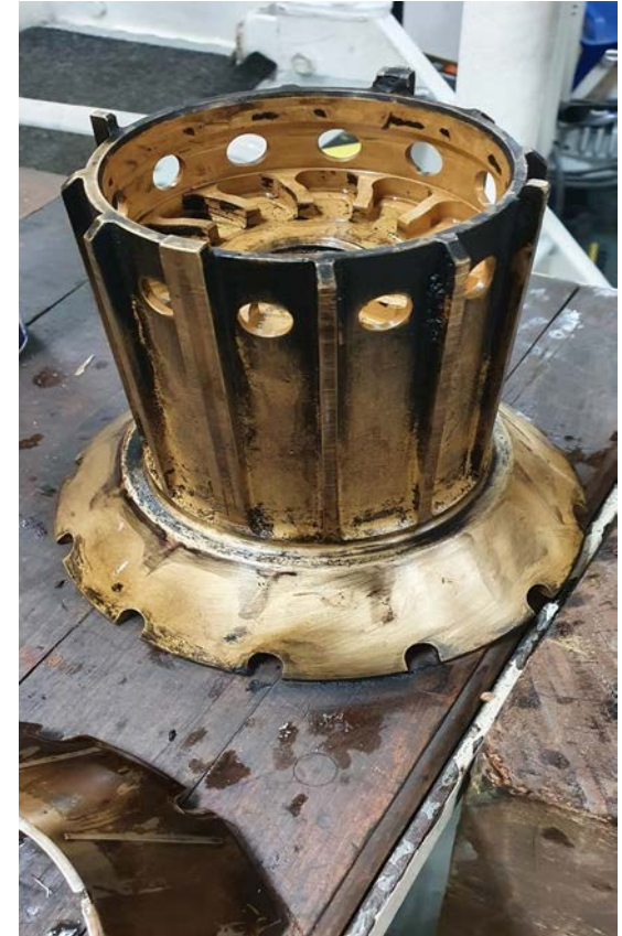
High Vol % presence of FAME impact on Bronze component
