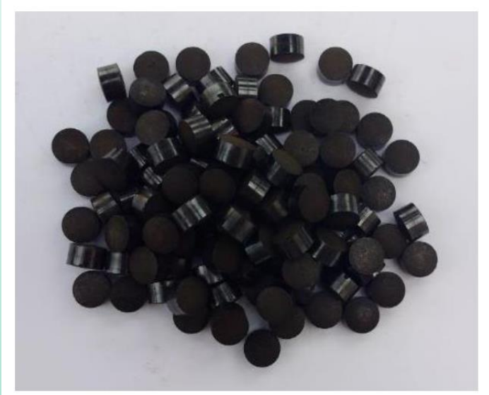
Typical methanol catalyst (Cu/ZnO/Al 2 O 3 ) in pellet form (Ø 4mm).
